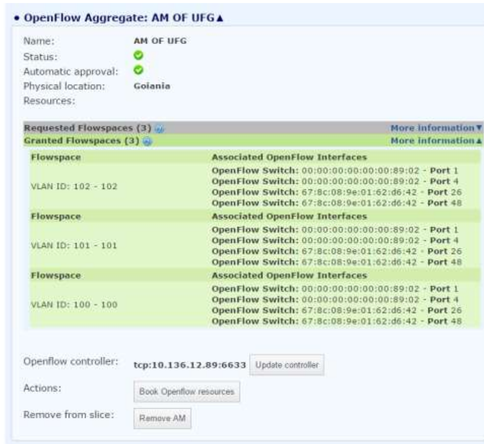
Figure 4. OpenFlow Aggregate area.
